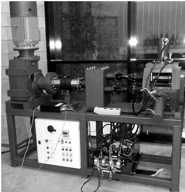
Fig. 10. Forging machine for rotary compression.
