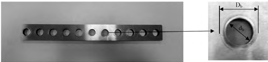
Fig. 2. The plate used in tightening tests ( d_h – clearance hole diameter and D_b – diameter of bearing surface).
