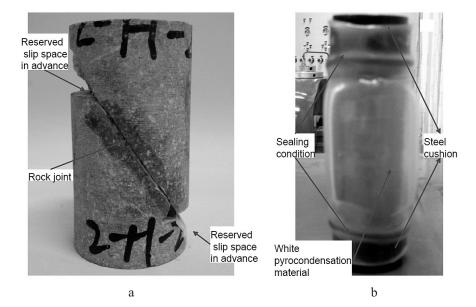
Fig. 2. Preparation for the tested specimen: (a) reserving sliding displacement space cut by a diamond saw in advance; (b) wrapping with heat shrink films to prevent hydraulic oil into rock joint fissure.
