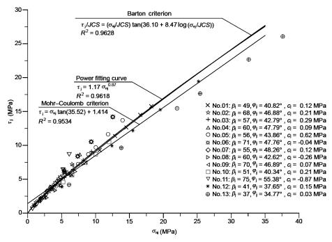
Fig. 5. The scatter point distribution in the  $\sigma_{nj} - \tau_j$  space and its fitting by three functions. ISSN 0556-171X. Проблемы прочности, 2015,  $N \ge 1$
