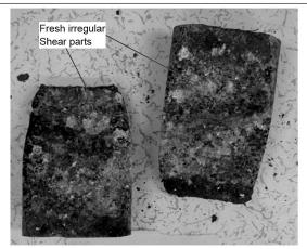
Fig. 4. The fresh irregular shear parts on the rock joint plane.
