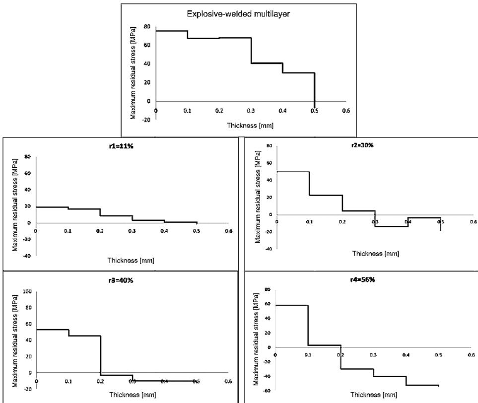
Fig. 4. Through-depth residual stress in explosive-welded and cold-rolled multilayers.
