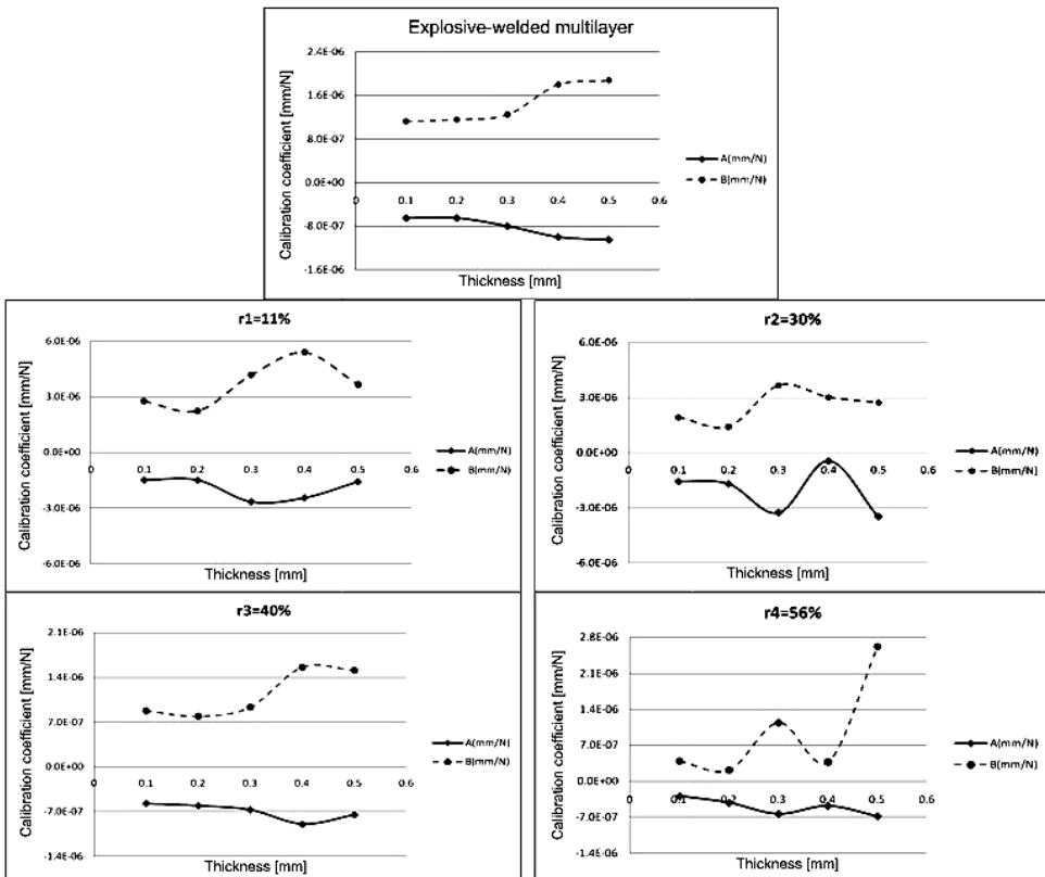
Fig. 3. Through-depth calibration coefficients in explosive-welded and cold-rolled multilayers.
