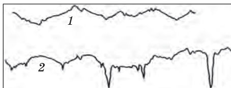
Fig. 23. The surface profilogram of the 9XC (HRC 32–64) samples processed by sharpening: 1 — MPP, 2 — in the water with addition of cooling lubricants [21]
