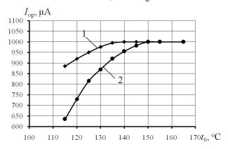
Fig. 7. Dependencies of the optical probe current, in the visible part of the light spectrum in the neutral and BIcharged steam flow, from its initial temperature at an initial pressure of 142.2 kPa:
