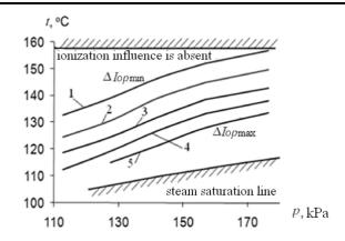
Fig. 9. Steam ionization efficiency depending on changes in pressure and temperature:
