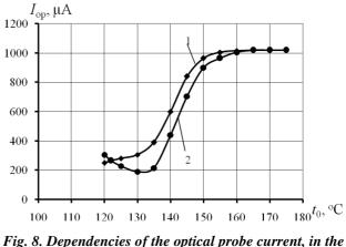
Fig. 8. Dependencies of the optical probe current, in the visible part of the light spectrum in the neutral and BIcharged steam flow, from its initial temperature at an initial pressure of 176.5 kPa:
