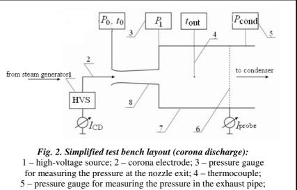
6 – grid (electric probe); 7 – exhaust pipe (zone of sudden expansion); 8 – nozzle
