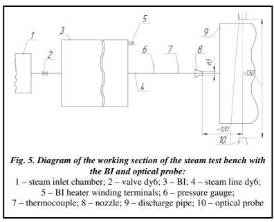
During the experiments in all the operating modes of the test bench, the values of the optical probe current of neutral and charged steam flows were recorded at different values of the initial temperature at the nozzle entry.
