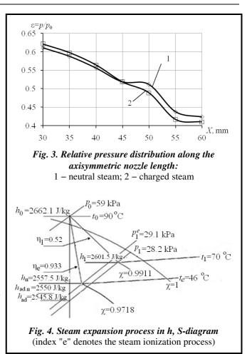
which forms, in the volume of steam,numerous hydrated ions (additional nuclei of heterogeneous condensation), which are a complex of an ion and water molecules linked to it by electrostatic forces. They become "frozen" in the steam flow, and, when falling into the volume of saturated and supersaturated steam, intensify the condensation process, thereby reducing the supercooling process level.
