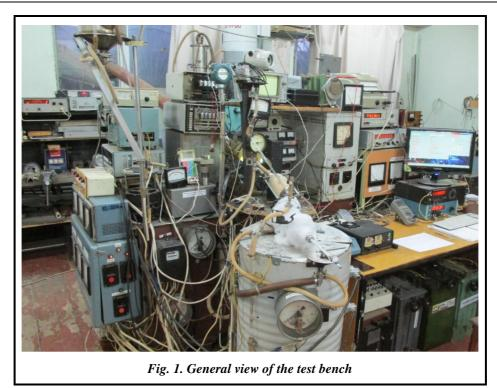
The steam generator provides the necessary steam flow rate of the following specified parameters: – absolute pressure from 30 to 110 kPa;
