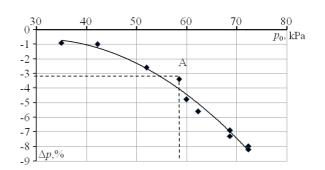
Fig. 10. Relative pressure change at the nozzle exit against the initial pressure
