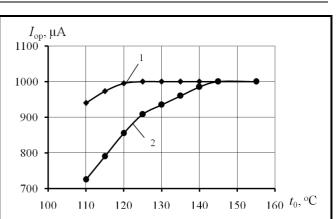
Fig. 6. Dependencies of the optical probe current, in the visible part of the light spectrum in the neutral and BIcharged steam flow, from its initial temperature at an initial pressure of 112.8 kPa:
