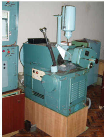
1 – rubber roller; 2 – abrasive material; 3 – mechanism of load creation; 4 – a sample of the studied material
