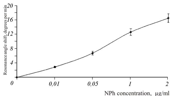
Fig.2 Response of the immune sensor to the introduction of different concentrations of NPh into the measuring cell with preliminary modification of the sensor surface with PAA/protein A/antiserum
