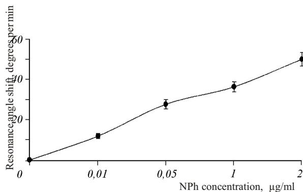
Fig.3 Response of the immune sensor to the introduction of different concentrations of NPh into the measuring cell with preliminary modification of the sensor surface with dodecanethiol
