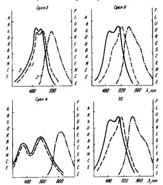
Absorption spectra profiles of free dyes and absorption and fluorescent emission spectra profiles of DNA - dyc complexes in TE: absorption patterns of free dyes (1), absorption (2) and the fluorescent patterns (3) of DNA - dyc complexes
