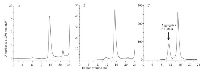
Fig. 3. Analysis of the full-length His-eEF1B $\gamma$  by gel filtration on Superose 6 HR column. Concentration of His-eEF1B $\gamma$  applied on column was: A-0.3 mg/ml; B-1.6 mg/ml; C-8 mg/ml
