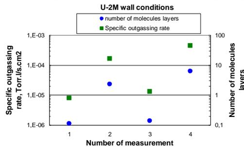
Fig. 7. U-2M wall conditions in different times of measurements: points with index 1 (RF) and 3 (VHF) were measured for standard procedure of discharge cleaning just after 18 hours pumping; points 2 and 4 were obtained one hour shortly after the discharge cleaning end both for the VHF(2) or RF(4)
