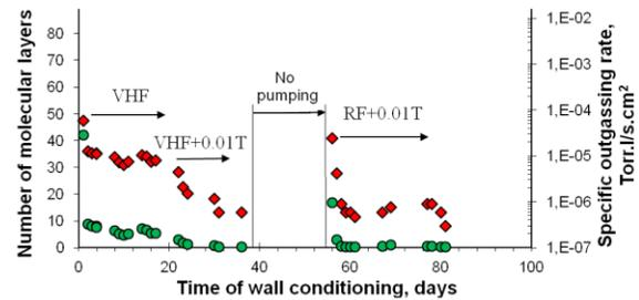
Fig. 6. Uragan-2M wall conditions: green points correspond to number of molecular layers on the surface of SS probe; red rhombs correspond to SS probe outgassing rate at  $300^\circ\text{C}$  after VHF or RF discharge cleaning and pumping
