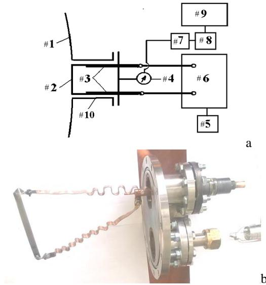
Fig. 1. The scheme of the experiment (a) and photo of device (b): 1 – U-2M vacuum chamber wall; 2 – stainless steel probe; 3 – current contacts; 4 – pressure gauge; 5 – time relay; 6 – electric power supply; 7 – VIT-2 vacuum measurement device; 8 – interface module WAD-AIK-BUS; 9 – computer; 10 – branch pipe
