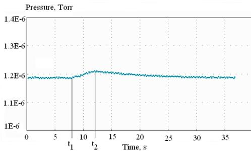
Fig. 3. Apparatus curve of pressure increase in the U-2M during SS probe heating to the temperature of  $300^\circ\text{C}$  after 1 minute of the first pulsed heating:  $t_1$  and  $t_2$  are the times of switch on and switch off the heating
