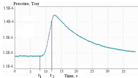
Fig. 2. Apparatus curve of pressure increase in the Uragan-2M during SS probe heating to the temperature of 300°C:  $t_1$  and  $t_2$  are the times of switch on and switch off the heating, initial pressure is  $1.18 \cdot 10^{-6}$  Torr
