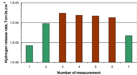
Fig. 8. Hydrogen release from the SS probe: green color – sample temperature under the measurement was 500°C; brown color – sample temperature under the measurement was 600...700°C
