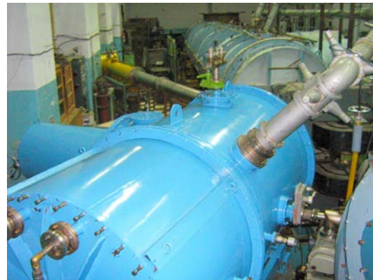
Fig. 2. Helium ions linac with an output energy of 4 MeV (foreground). Main section of the multicharged ions linac (background)
