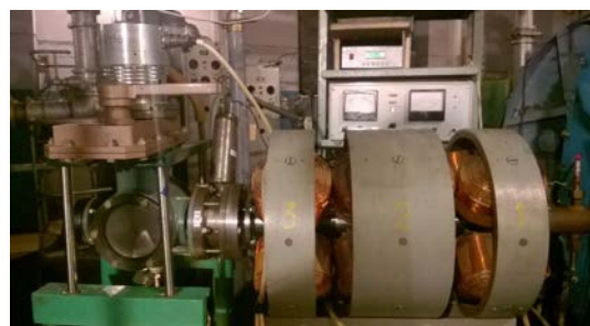
Fig. 3. Transport line for the helium ions beam. Left to right: irradiation chamber with samples, focusing triplet, output of the accelerator
