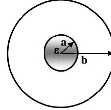
Fig. 2. Geometry of the dielectric coaxial line
