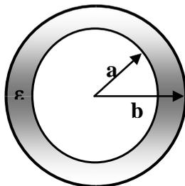
*Fig. 1. Tubular dielectric waveguide*
