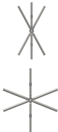
Fig. 8. Example of RF field tuning on the model structure with CRFF for the focusing period FOOODDOOOF: a) the shafts are swung 110^\circ to either side of initial position (left) and corresponding distribution of E_z component of the RF field along the accelerating structure (right); for a corner of bars turn concerning initial position in IH structures on \pm 110^\circ and distribution E_z component of RF field along accelerating structure; b) the rotation angle is \pm 160^\circ (left) and corresponding E_z distribution (right)
