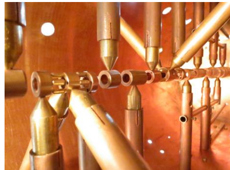
Fig. 7. General view of the model for accelerating and focusing channel with CRFF with adjusting elements
