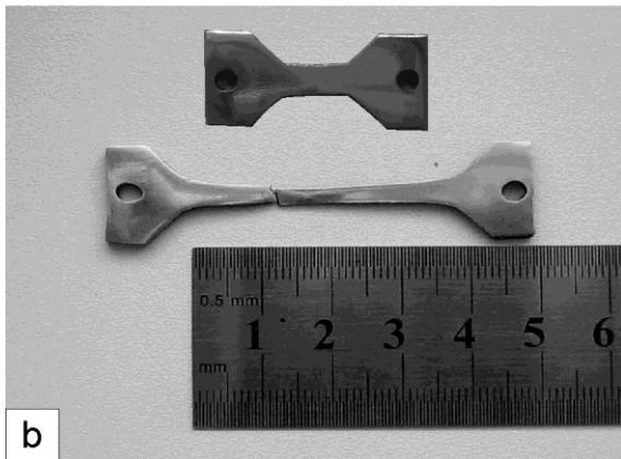
Fig. 1. Elongation to failure \delta , as a function of the test temperature T for the Al-Zn-Mg-Cu-Zr alloy (a), the general view of the initial specimen and a view of the specimen deformed to failure under the optimal conditions (b)
