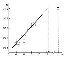
Fig. 1. Dependence of the face area perpendicular to the c axis, S=ab ( $\mathring{\rm A}^2$ ), on the number of the perovskite-like layers in the structure of  ${\rm Bi}_{m+1}{\rm Fe}_{m-3}{\rm Ti}_3{\rm O}_{3m+3}$  compounds (1 – Aurivillius phases; 2 –  ${\rm BiFeO}_3$ ).
