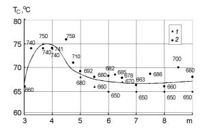
Fig. 2. Dependence of the Curie temperature on the number m (1- DTA data; 2 - DSC ones).
