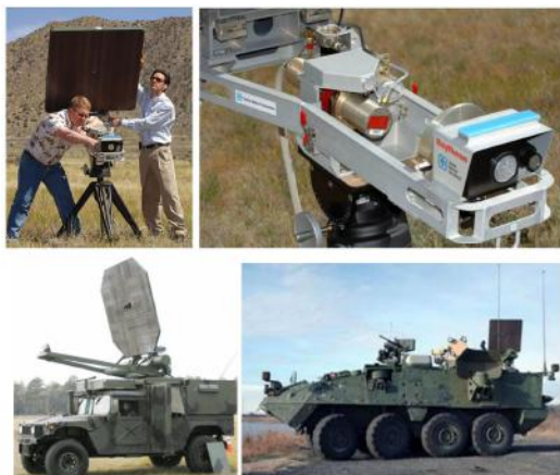
Fig. 6. Compact source of powerful monodirectional ultra-shortwave radiation (95 GHz) developed by Sandia National Laboratories, USA, under Raytheon technology (top), and powerful sources of mono-directional radiation assembled on chassis of Hummer off-roadster and ACP Stryker. More powerful complex is planned to be installed on board of AC-130 airplane
