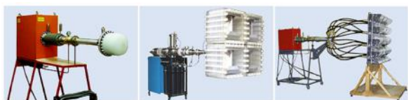
Fig. 5. Compact powerful ultra-wideband sources of radiation with capacity up to 1 GW developed at Tomsk Institute of High Current Electronics
