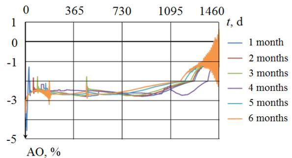
Fig. 3. Axial offset dependence on time for WWER-1000 power control program III
