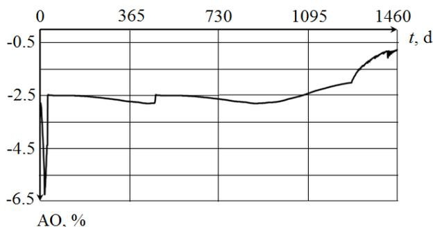
Fig. 2. Axial offset dependence on time for WWER-1000 power control program II
