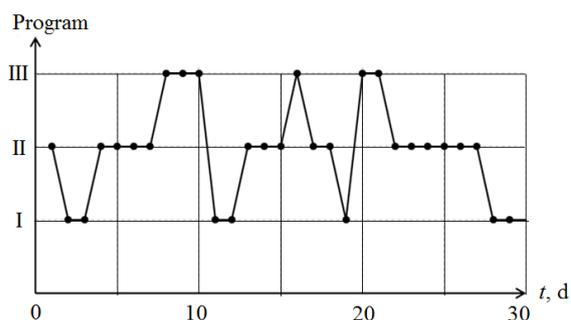
Fig. 6. Schedule of transitions between power control programs for one month of power maneuvering
