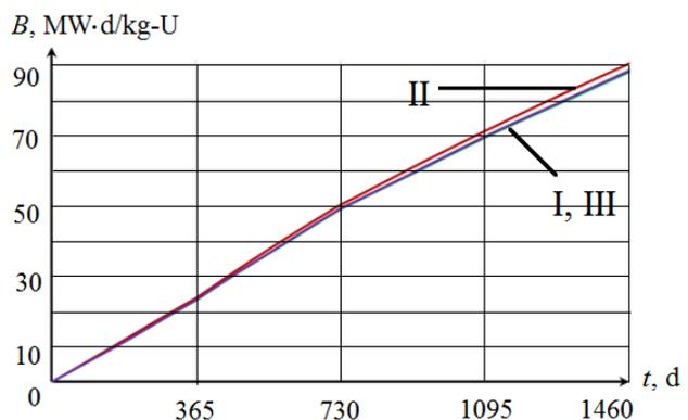
Fig. 4. Burn up dependence on time for WWER-1000 power control program I ( $\langle t_w \rangle = \text{const}$ ), II ( $p_2 = \text{const}$ ), and III ( $t_{w,0} = \text{const}$ )
