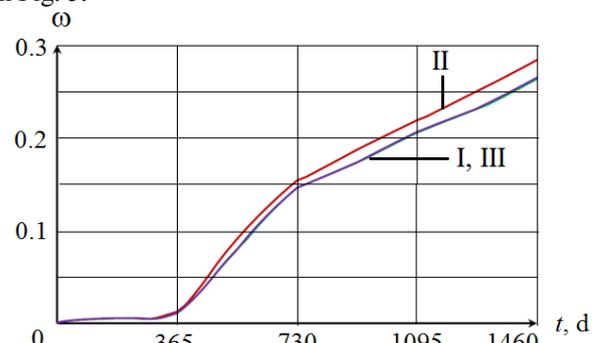
Fig. 5. Cladding damage parameter dependence on time for WWER-1000 power control program I ( $\langle t_w \rangle = \text{const}$ ), II ( $p_2 = \text{const}$ ), and III ( $t_{w,0} = \text{const}$ )
