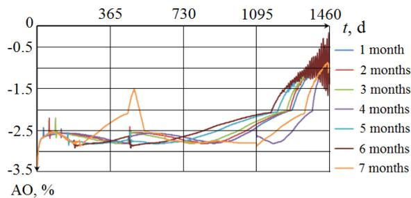
Fig. 1. Axial offset dependence on time for WWER-1000 power control program I
