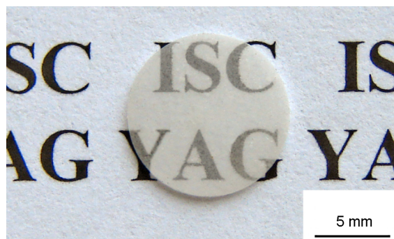
Fig. 7. 1 mm thick Y_3Al_5O_{12} ceramics sintered in vacuum at 1750°C for 20 h.
