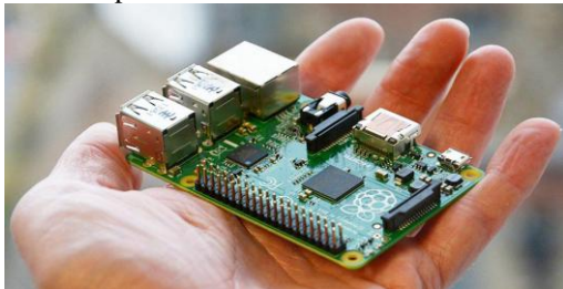
Fig. 3. The picture of a single-board mini computer Raspberry Pi-3
