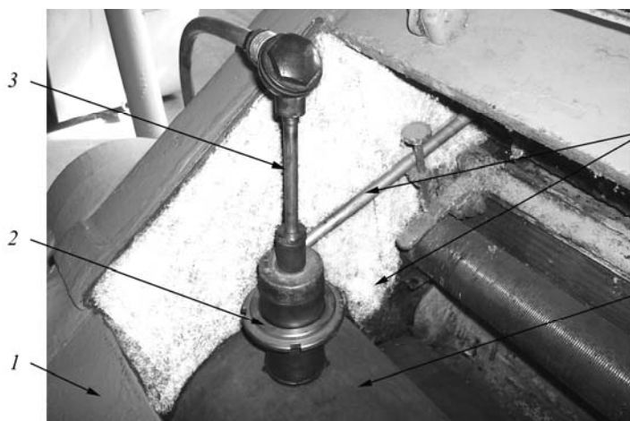
Fig. 2. Device for temperature measuring on smooth cylindrical surfaces: 1 – roller mill; 2 – body of the unit; 3 – thermocouple (ТХА-775); 4 – fasteners device; 5 – cylindrical roller.
