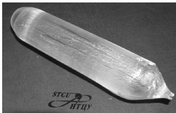
Fig. 2. GSO crystal grown using the additional heating during the final stage of the crystal formation.
