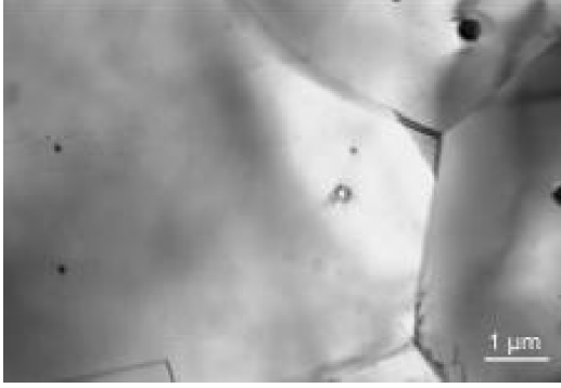
Fig. 1. The initial microstructure of SS316 steel after heat treatment at 1050 °C/0.5 h
