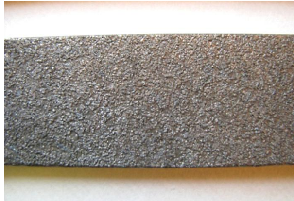
Fig. 4. The appearance of the sample surface hardened by steel 15X11MΦIII.
