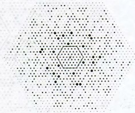
Fig. 3. 24-element nonredundant configuration on the hexagonal grid of radius r = 10 and the coverage of the u, v -plane. The large dots represent the configuration elements while the small ones – the baselines in the u, v -plane. The inner, element-free domain of radius r_0 = 4 is singled out
