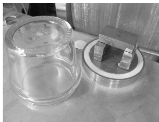
Fig. 2. Working chamber of the experimental installation to form coating by aerosol deposition method.
