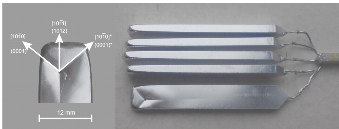
Fig. 3. Five Zn bicrystals (photo) grown simultaneously from one single-crystal seed. The bicrystal turned by 90^\circ was indented to visualize the longitudinal grain boundary trace and two traces corresponding to (0001) planes of each grain.
