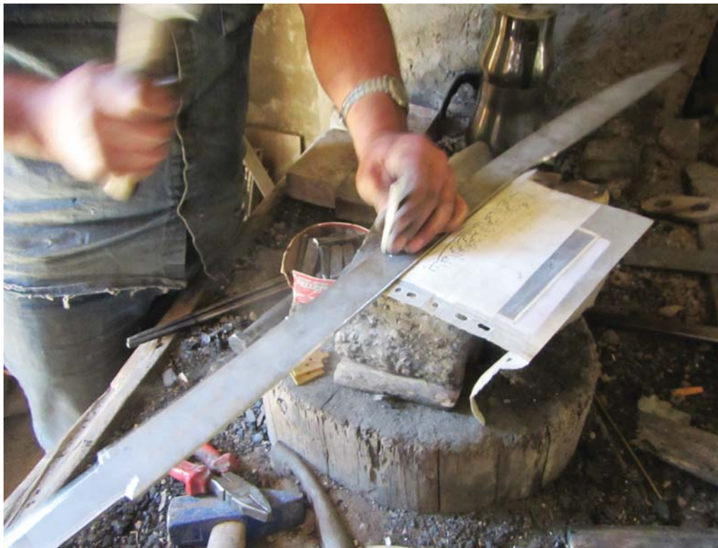
Fig. 5. Using a stamp to create the recess.
