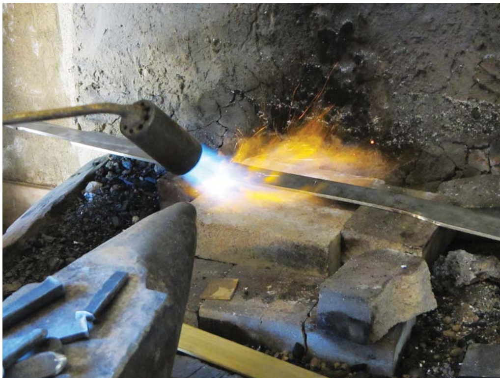
Fig. 6. Melting the brass inlay so it fills the recess.
