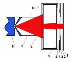
Fig. 2. Scheme of hydrogen negative ion beam current measurement at 8 cm distance from the source aperture: 1-5) collectors for measurements of the beam current components; 6) hydrogen negative ion beam;
