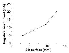
Fig. 7. Dependence of current onto remote collector from the source with anode holes of 2, 3.5, and 4 mm diameter on output slit surface. Pulsed discharge power is 15 kW
