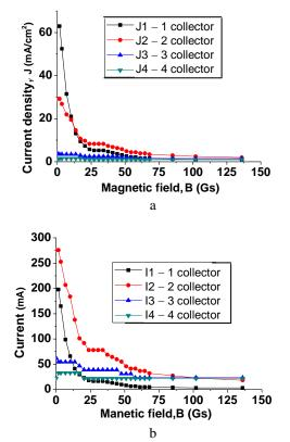
Fig. 4. Dependence of current density onto collectors on magnetic field strength. The discharge current is 30 A (a); Plot of averaged total current onto lamella obtained by multiplying the current density by each lamella area (b)
