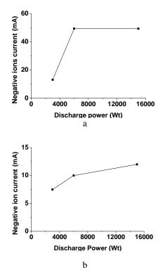
Fig. 5 Dependencies of total negative ion current with  $14^{0}$  propagation angle at 8 cm distance from the source aperture (a) and hydrogen negative ion current with  $12^{0}$  propagation angle at 50 cm distance from the source (b) on power introduced into the discharge
