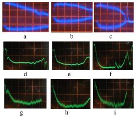
Fig. 3. Oscillograms of the discharge parameters of the source of negatively charged particles (a-c), and current values onto central electrode of modernized collector at turned off (d-f), and on (g-i) transverse magnetic field. (a-c) the top trace represents the discharge voltage, 50 V/div (a), 100 V/div (b,c); (a-c) the bottom trace represents the discharge current, a)
