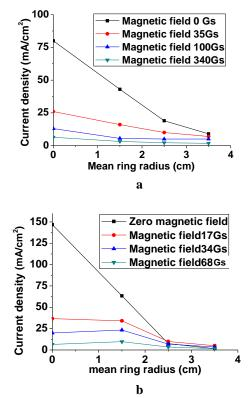
Fig. 6. Distributions of negative hydrogen ion beam current density over the rings of combined collector for different magnetic field strength and emission slit aperture 4 mm (a) and 3.5 mm (b). Pulsed discharge power is 15 kW
