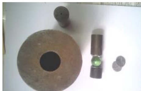
Fig. 2. High pressure cylinder with the embedded simulation glass specimen
