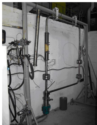
Fig. 3. Loop2 on the test bed. The arrow specifies a placement of the flow monitor
