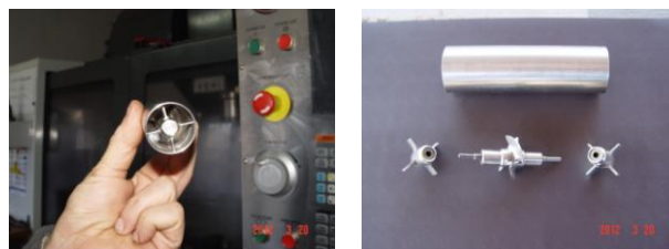
Fig. 2. An external view of the monitor N1 for the control of the water flow in SCWCL
