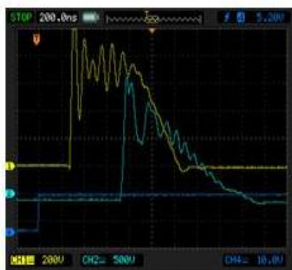
Fig. 2. Pulses on thyatron grids from trigger unit MA2709A
