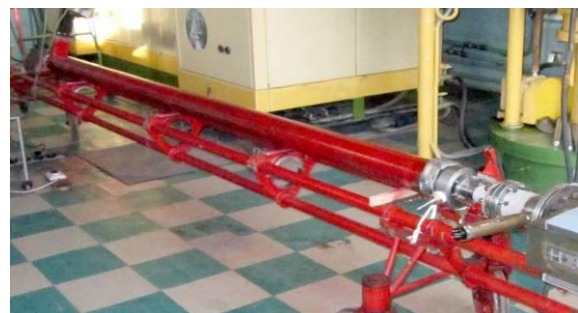
Fig. 15. Photo of the section on the frame (section is under vacuum)
