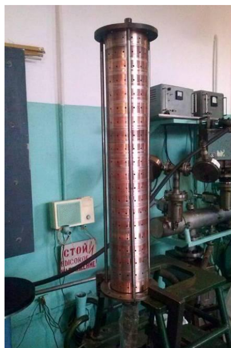
Fig. 4. Vacuum testing of subsection on helium leak detector
