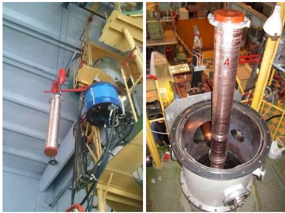
Fig. 5. Loading of the fourth subsection into the induction vacuum furnace, subsection is in chamber (output coupler is not brazed)
