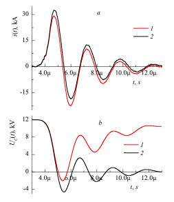
Fig. 3. The dynamics of the discharge current (a) and the dynamics of the capacitor bank discharge (b) for the observed (1) and restored (2) signal
