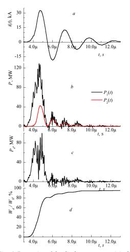
Fig. 4. Dynamics of the discharge current (a), the total active power in the circuit (b), the additional active power released in the discharge (c) and the absorbed energy (d)
