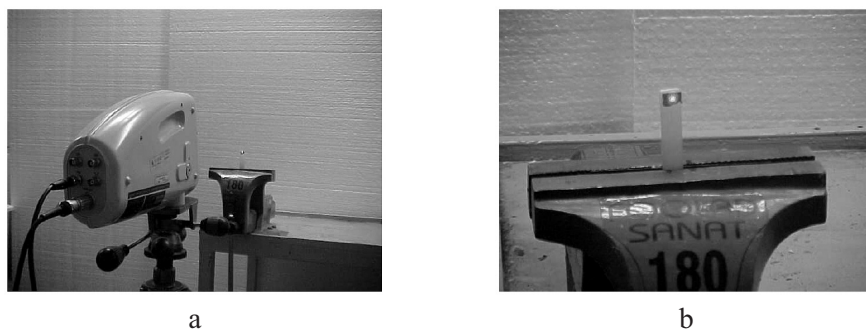
Fig. 1. Vibration measurement by laser doppler vibrometer OMETRON VH300+ (a) and specimen (b).
