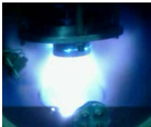
Fig. 11. Plasma jet in high-current mode
