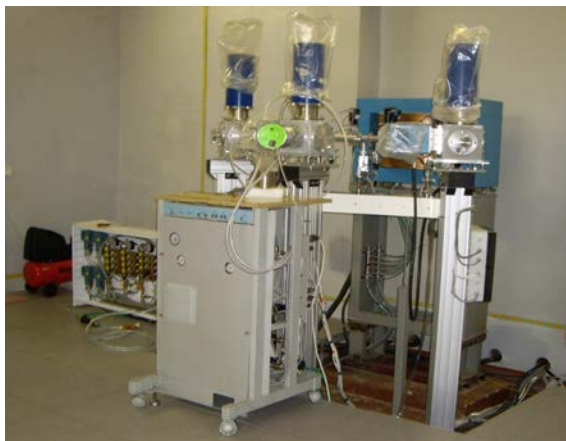
Fig. 6. Cabinet of the target control system n in the target hall of the cyclotron
