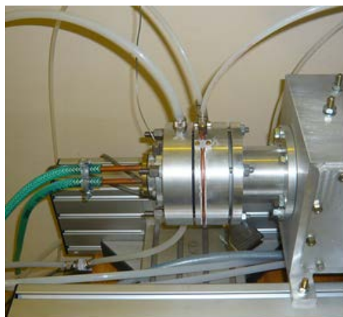
Fig. 2. The target device for ^{18}\text{F} production
