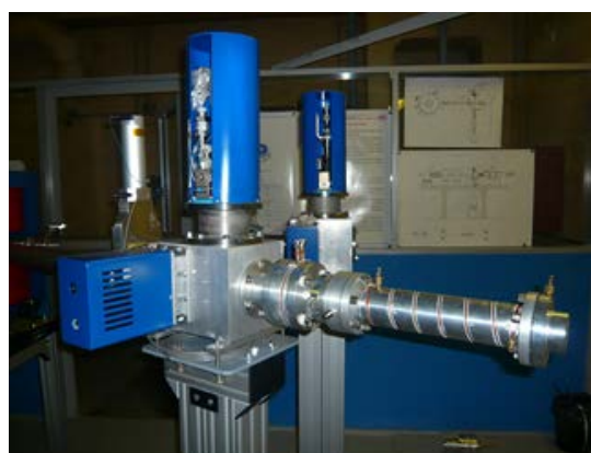
Fig. 5. The target device for ^{11}\text{C} production
