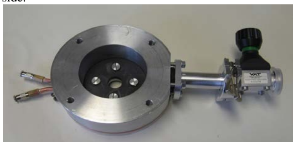
Fig. 3. Water-cooled collimator unit
