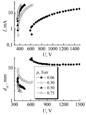
Fig. 2. Discharge current and cathode sheath thickness against voltage for different N<sub>2</sub>O pressure values and the inter-electrode distance of 20 mm
