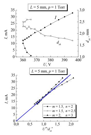
Fig. 4. Discharge current and cathode sheath thickness against voltage for the  $N_2O$  pressure of 1 Torr and the inter-electrode distance of 5 mm, as well as discharge current against the  $U^m/d_{sh}^n$  ratio values (m = 1.5, n = 2; m = 1.5, n = 2, 5; m = 2, n = 3)
