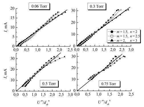
Fig. 3. Discharge current against  $U^m/d_{sh}^n$  ratio (m = 1.5, n = 2; m = 1.5, n = 2,5; m = 2, n = 3) for different N<sub>2</sub>O pressure values. Inter-electrode difference is 20 mm
