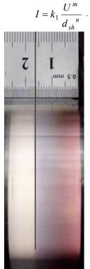
Fig. 1. Discharge photo for the inter-electrode distance of 25 mm, the  $N_2O$  pressure value of 0.05 Torr and the current value of 4.6 mA. The line indicates the location of the cathode sheath boundary
