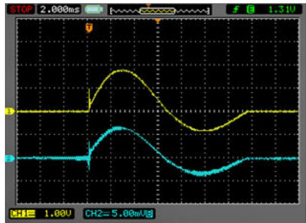
Fig. 4. Oscillograph of the cylindrical magnetic field solenoid current measured with the help of shunt (1) and Rogowski loop (2)
