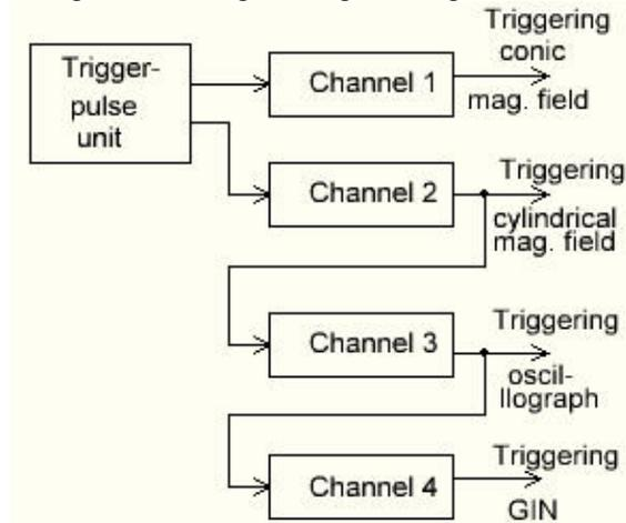
Fig. 5. Block diagram of the synchronizer
