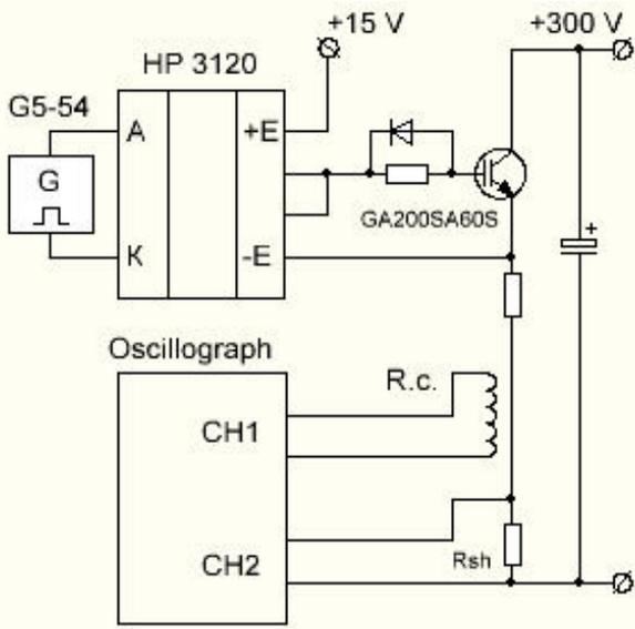
Fig. 3. Schematic representation of the stand for Rogowski loop calibration
