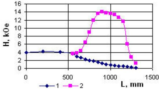
Fig. 1. Magnetic field distribution along the accelerating column axis
