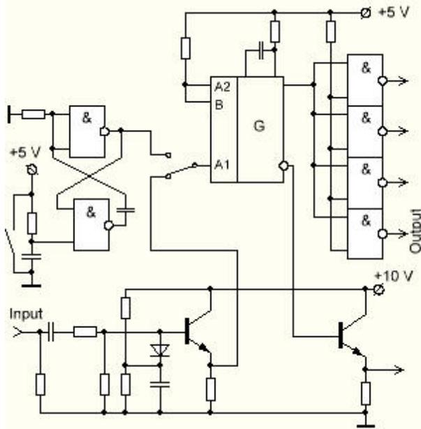
Fig. 6. Schematic representation of the trigger-pulse unit
