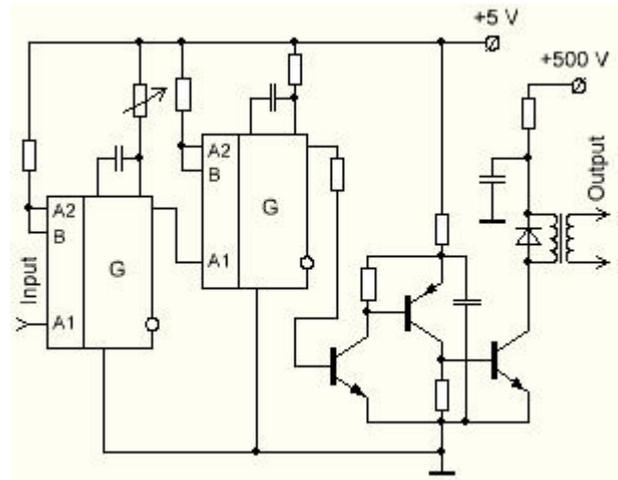
Fig. 7. Schematic representation of the delay unit
