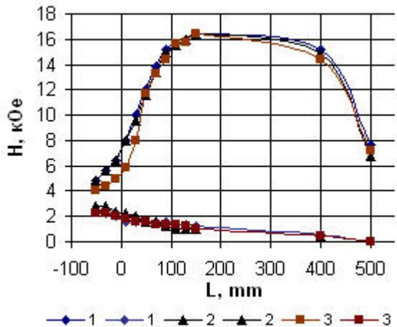
Fig. 2. Magnetic field strength distribution along the cylindrical field radius
