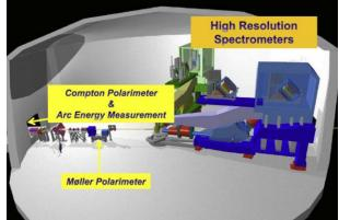
Fig. 4. Layout of Hall A showing the existing pair of High Resolution Spectrometers and polarimeters being upgraded
