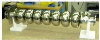
Fig. 2. Cavity of new Cryomodule C-100
