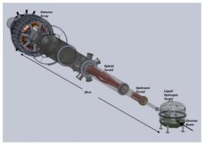
Fig. 6. Layout of MOLLER experiment equipment in Hall A
