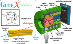
Fig. 10. Layout of detector Glue-X in new hall D
