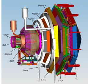
Fig. 8. Schematic of CLAS12 – a new spectrometer in Hall B
