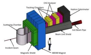
Fig. 5. Layout of new spectrometer SBS (Super Big Bite) in Hall A
