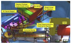
Fig. 9. Layout of Hall C after reconstruction. The existing HMS detector and a new detector SHMS are shown
