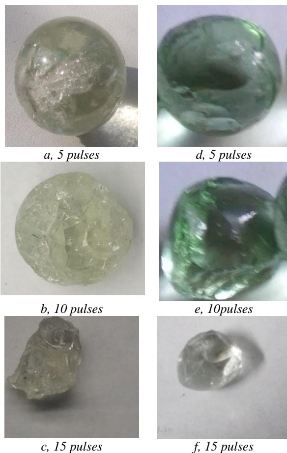
Fig. 4. Specimen milling steps: a, b, c – grinding by way of crushing; d, e, f – grinding by way of the cleavage
