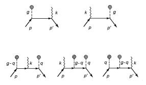
Feynman diagrams corresponding to the first and the second Born approximations in the description of bremsstrahlung in the external field
