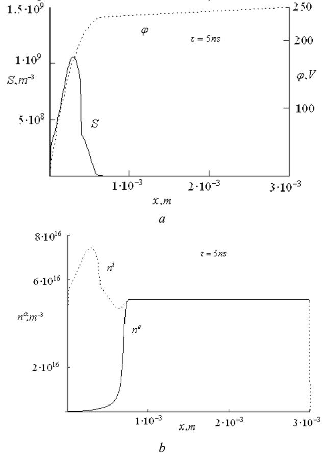
Fig.2. a – spatial distribution of potential and ionization-recombination source; b – spatial distribution of electron and ion densities.  $t=5 \text{ ns}$ , other parameters are the same as on Fig.1
