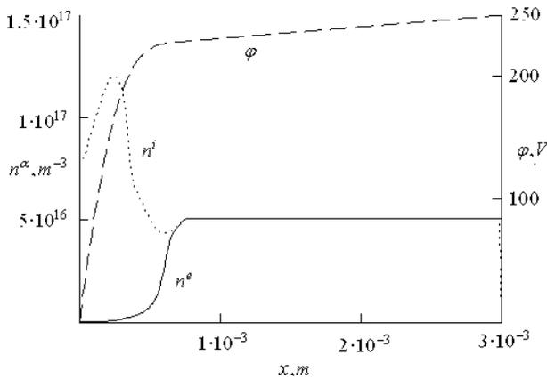
Fig. 1. Spatial distribution of potential and electron and ion densities for glow discharge in nitrogen ( $p=1995 \text{ Pa}$ ,  $T=300\text{K}$ ,  $\gamma=0.33$ ,  $E=250 \text{ V}$ )
