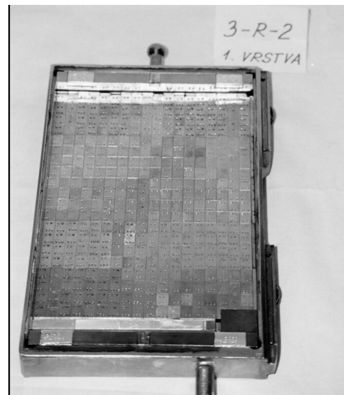
Fig. 4. Container of the Modified/Integrated Surveillance Program with inserts
