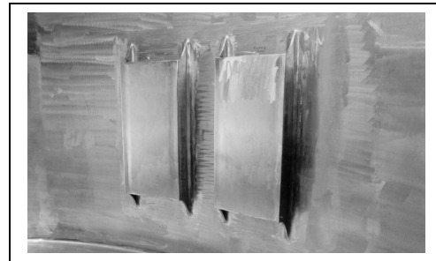
Fig. 3. Container of the Modified/Integrated Surveillance Program in NPP Temelin
