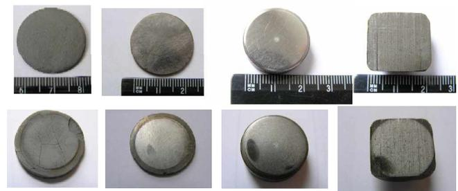
*Fig.1. The HPV W on Ni substrate, (W-1% Ni), HPV (W-5% Cu), HPV (W-5% Cu) after Cu evaporated (all above). All samples at the foot are after exposure to plasma*
