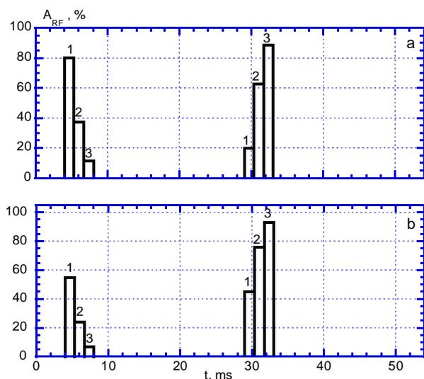
Fig. 5. Distribution of averaged harmonic amplitudes between the breakdown stages (4 to 9 ms) and the quasi-stationary stage of the discharge (9 to 54 ms): a) upper half-plane; b) lower half-plane
