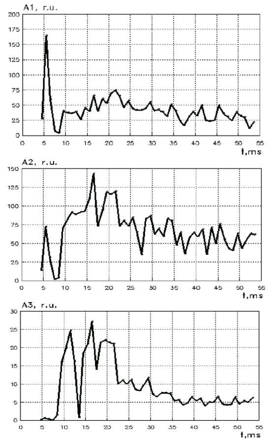
Fig. 4. Behavior of RF field harmonic amplitudes during the discharge (channel 1)
