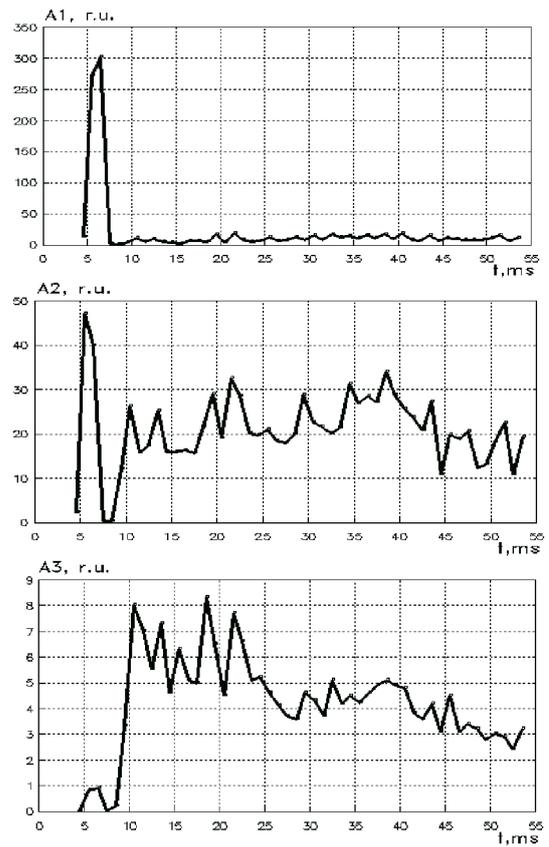
Fig. 3. Behavior of RF field harmonic amplitudes during the discharge (channel 2)
