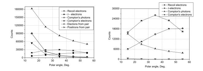
Fig.4. The angular dependence of the particles yields from main QED processes and the  $\delta$ -electron production. Photon energy is  $E_{\gamma} = 100 \, MeV$  (left panel) and 1000 MeV (right panel), target is the plastic  $0.5 \,mm$ . Number of photons  $5 \cdot 10^9$ . The points present sum of the particles yield of the corresponding processes in the  $\pm 5^{\circ}$  angular intervals
