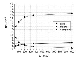
**Fig.2.** The yield of the QED processes on  $10^4$ photons as a function of the photon energy for plastic target of 1 mm thick. The recoil electron momentum  $q > q_0 = 0.1 \text{ MeV/c}$  were taken into account
