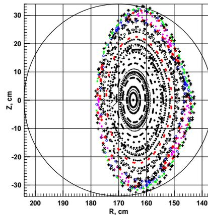
Fig. 9. Magnetic surface structure at the configuration mode with  $k_\phi=0.285$  and  $\langle B_\perp/B_0 \rangle=1.45\%$ : the mean radius of the closed magnetic surface, which is adjacent to a chain of magnetic islands with  $i/2\pi\approx 1/3$ , is  $a=20.5$  cm;  $\Delta=-5.3$  cm;  $i/2\pi(0)\approx 0.18$ ;  $i/2\pi(a)\approx 1/3$ ;  $\delta\approx 1.5-4.5$  cm; a large angular length of the islands
