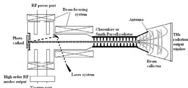
Fig.1. General layout of the THz generator
