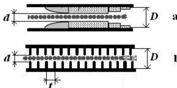
Fig.4. The conducting (metal) capillary coated inside by dielectric (a) and the corrugated channel or grating surface (b)
