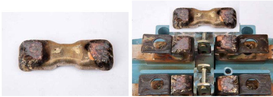
Fig. 16. View of used contacts Cu—Mo after 6000 switching cycles.
