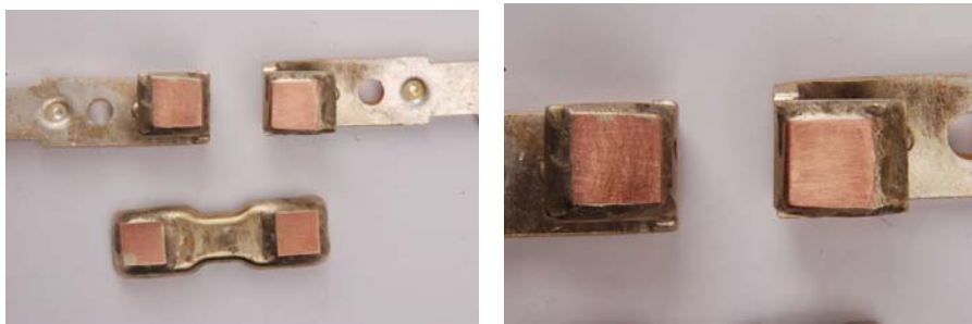
Fig. 12. View of new contacts made of composition Cu—Mo.
