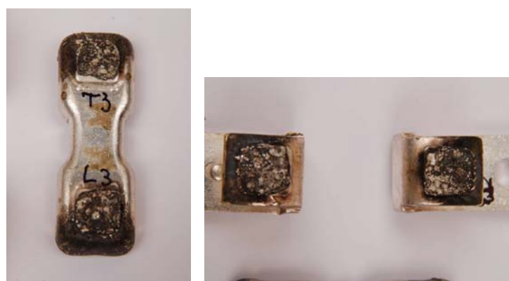
Fig. 10. View of used silver based contacts after 6000 switching cycles.
